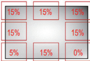
Segmentizing the areas and individual brightness control
