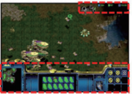
Local Brightness control with detecting static image area
